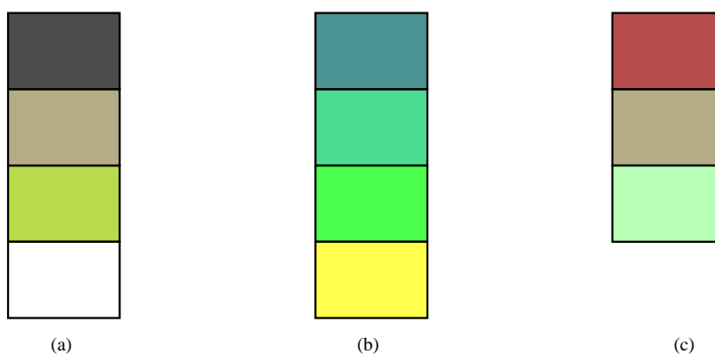
Figure 3. Representative clay horizons. Key: (a) Nakawa, Seta, Lwanda and Kajansi clays; (b) Umatengah, Chodah and Kumi clays; (c) Mutufu, Chelel, and Budadiri clay deposits.
