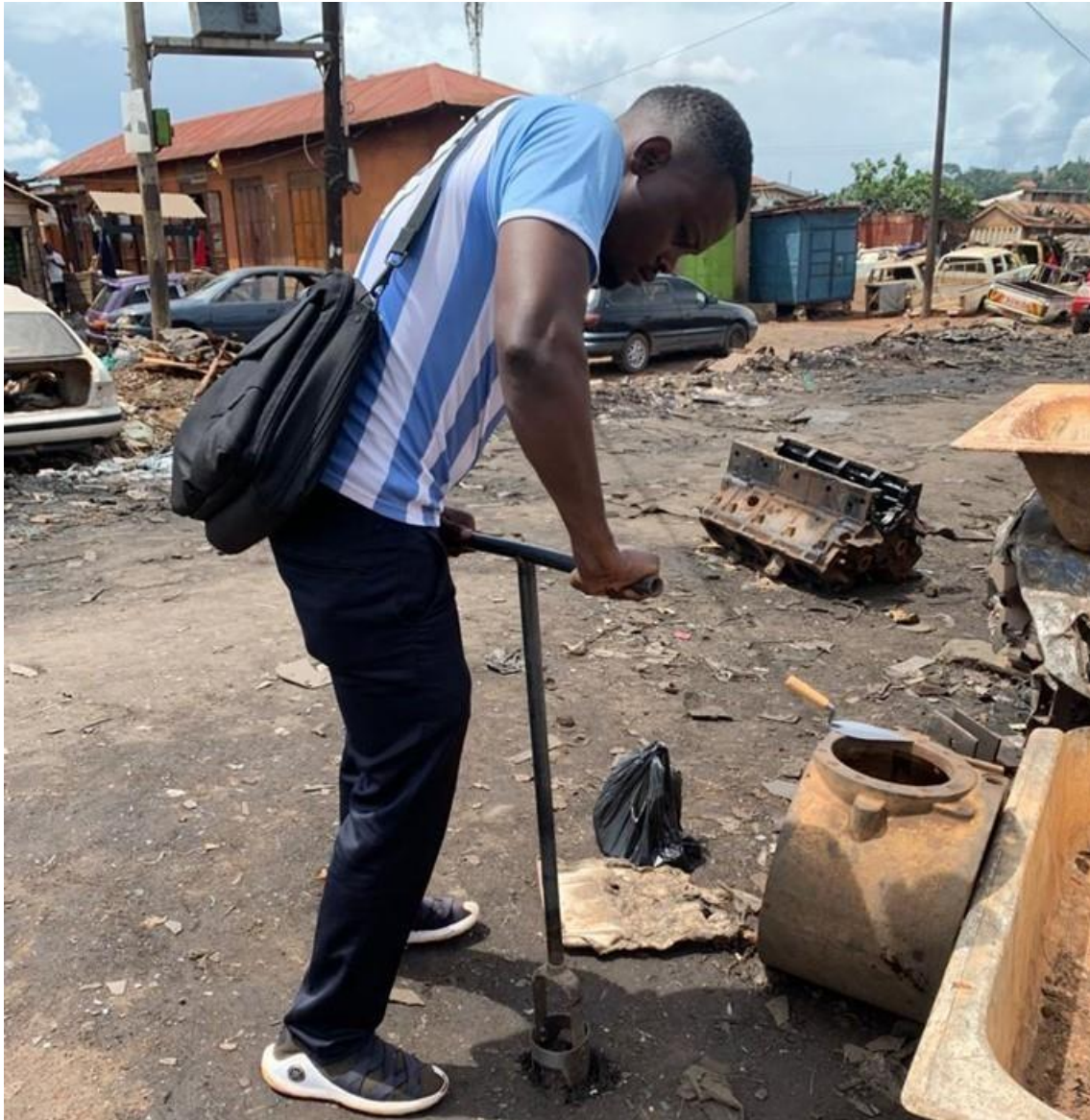
Figure 5: Utilizing a Hand-Operated Soil Auger to Extract Soil Samples
